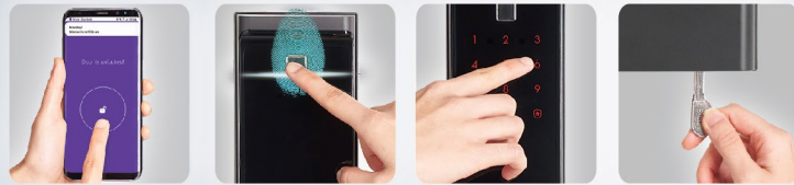
手機App(WiFi) Mobile App (WiFi) | 指紋 Fingerprint | 用戶密碼 User Access Code | 機械鎖匙(後備) Mechanical Override Keys
